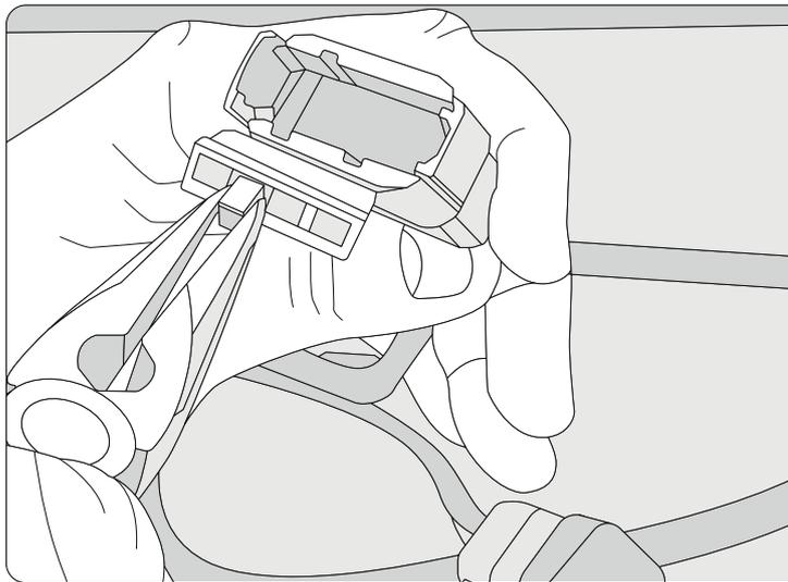
**1)** Take Connector 1 and remove the wedge lock.
